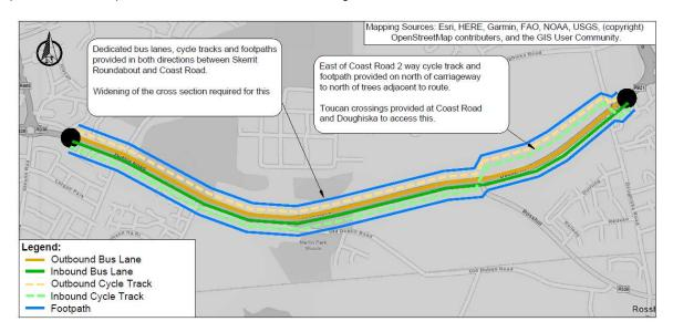
Figure 3-39 Section 2 Option 9 Indicative Scheme Design
