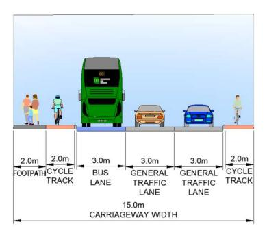
Figure 3-34 Section 2 Option 6D Indicative Cross Section
