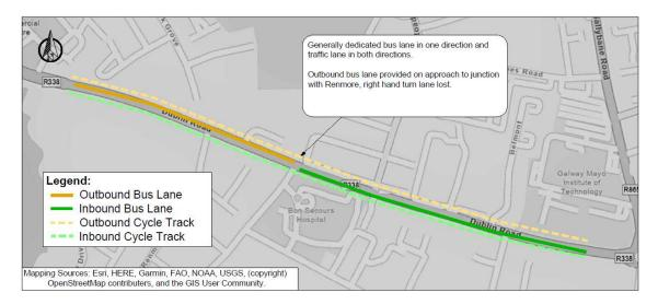
Figure 3-13 Section 1 Option 3 Indicative Scheme Design
