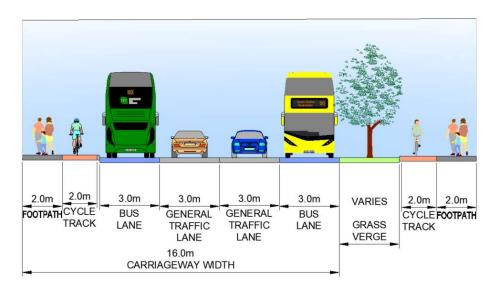
Figure 3-22 Section 2 Option 3 Indicative Cross Section
