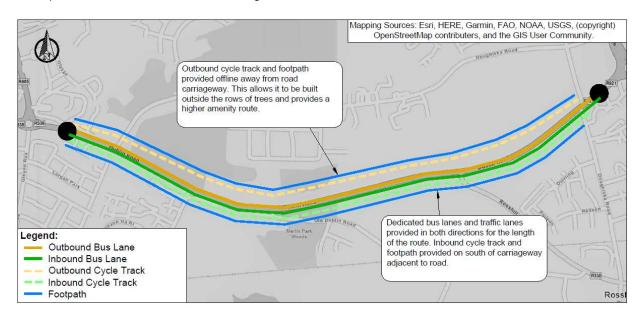
Figure 3-21 Section 2 Option 3 Indicative Scheme Design
