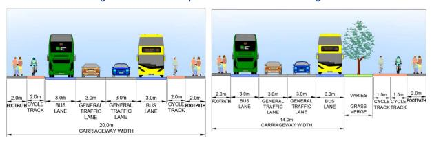
Figure 3-40 Section 2 Option 9 Indicative Cross Section
