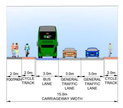
Figure 3-28 Section 2 Option 6A Indicative Cross Section
