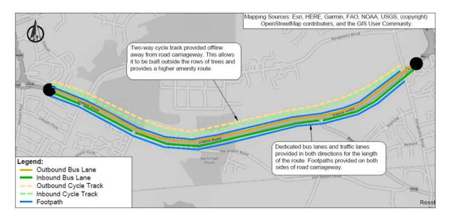
Figure 3-23 Section 2 Option 4 Indicative Scheme Design
