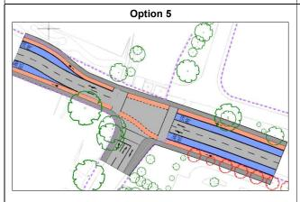
This option has the narrowest cross section of all options considered in this assessment. To reduce the amount of land take required the inbound bus lane is dropped for 30m after the junction, the bus lane is then picked up again after the pinch point. The outbound bus lane is also dropped 30m before the junction and a yellow box would allow outbound buses to enter the outbound traffic lane there. No dedicated right turn lane is provided for general traffic turning into Renmore Road.
