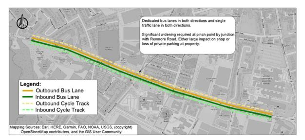
Figure 3-9 Section 1 Option 1 Indicative Scheme Design
