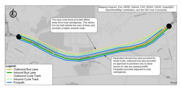
Figure 3-37 Section 2 Option 8 Indicative Scheme Design
