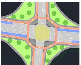
Due to the amount of space around the Skerritt Roundabout there would be room to upgrade the junction to the Cyclops style layout. This would allow bus priority to be controlled and provide priority for pedestrians and cyclists. By providing continuous bus, cycling and pedestrian infrastructure with signalised crossings this option would meet all 6 main objectives from the SAR.
