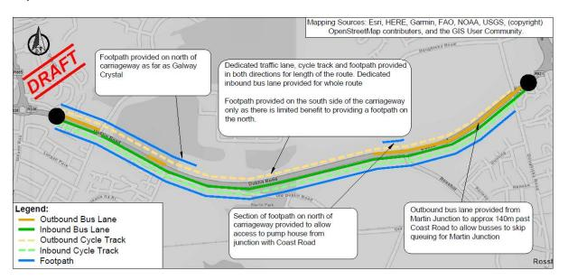
Figure 3-27 Section 2 Option 6A Indicative Scheme Design
