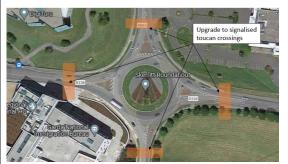
Upgrading the junction to provide signalised crossing would allow safe usage for pedestrians. By providing continuous bus, cycling and pedestrian infrastructure with signalised crossings this option would meet all six main objectives from the Strategic Assessment Report (SAR).
