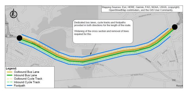
Figure 3-17 Section 2 Option 1 Indicative Scheme Design
