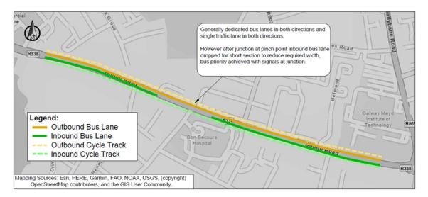
Figure 3-15 Section 1 Option 4 Indicative Scheme Design
