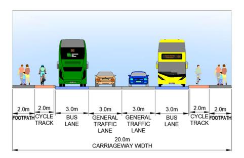
Figure 3-16 Section 1 Option 4 Indicative Cross Section
