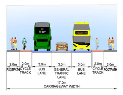
Figure 3-12 Section 1 Option 2 Indicative Cross Section
