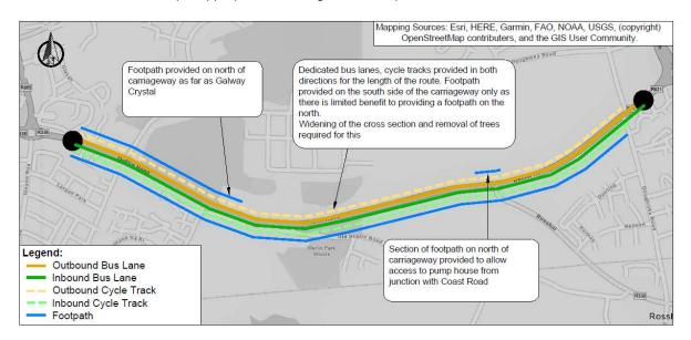
Figure 3-19 Section 2 Option 2 Indicative Scheme Design
