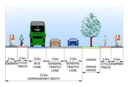
Figure 3-36 Section 2 Option 7 Indicative Cross Section
