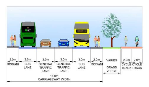
Figure 3-24 Section 2 Option 4 Indicative Cross Section
