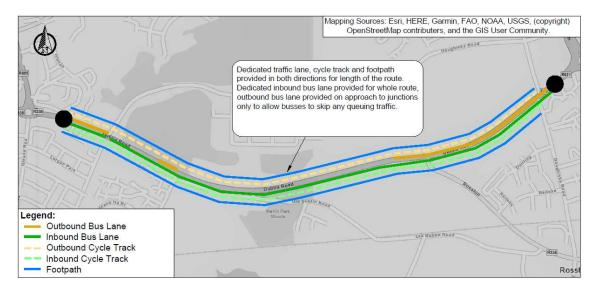
Figure 3-25 Section 2 Option 5 Indicative Scheme Design
