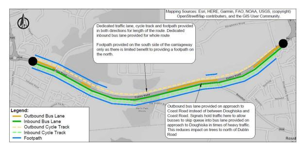
Figure 3-29 Section 2 Option 6B Indicative Scheme Design
