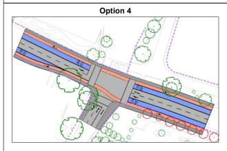
To reduce the amount of land take required this option has the inbound bus lane dropped for 30m after the junction. The bus lane is then picked up again after the pinch point. This option would also not have a dedicated right turn lane for general traffic.
