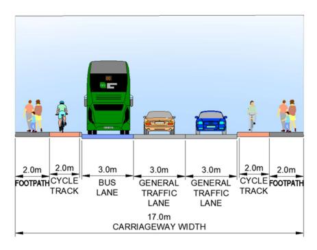
Figure 3-26 Section 2 Option 5 Indicative Cross Section
