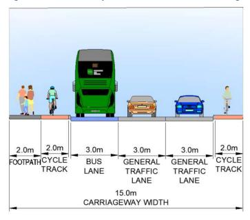
Figure 3-30 Section 2 Option 6B Indicative Cross Section
