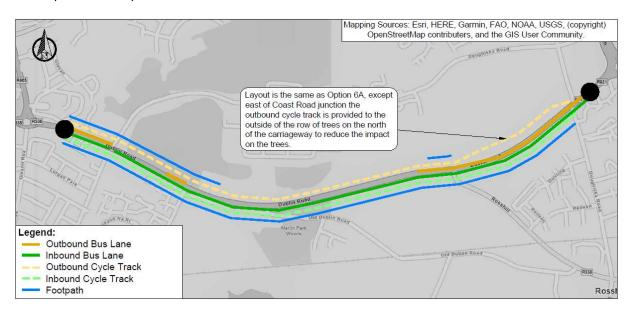
Figure 3-31 Section 2 Option 6C Indicative Scheme Design
